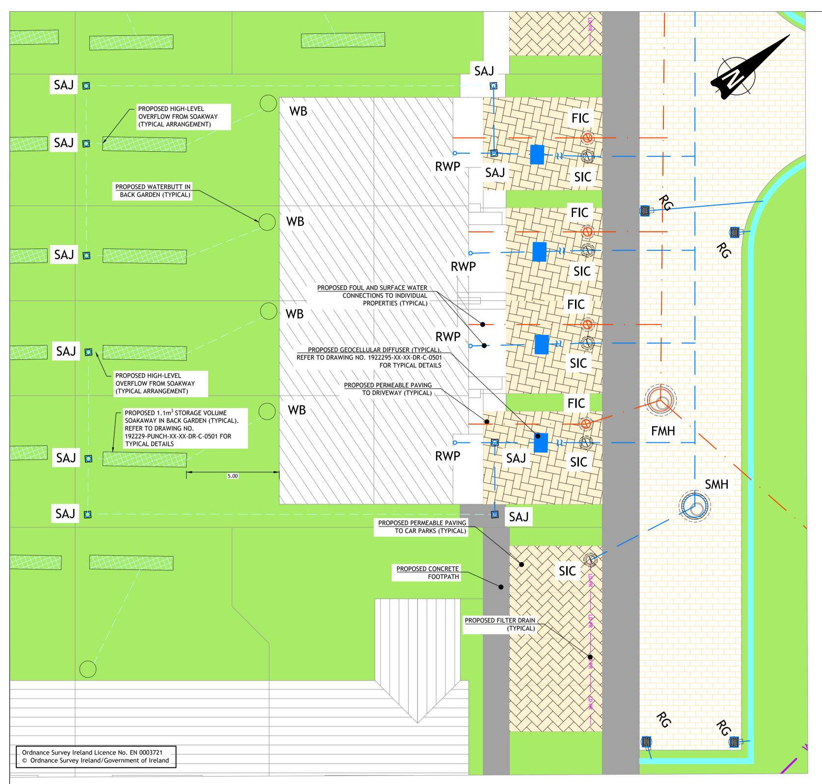
TYPICAL DRAINAGE ARRANGEMENT FOR INDIVIDUAL PROPERTIES
